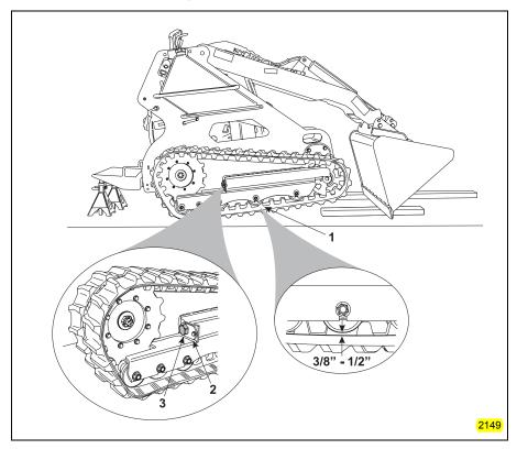
Figure 4–23 Track Tension Adjustment
